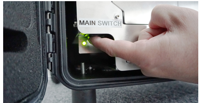
Main switch on the main unit
