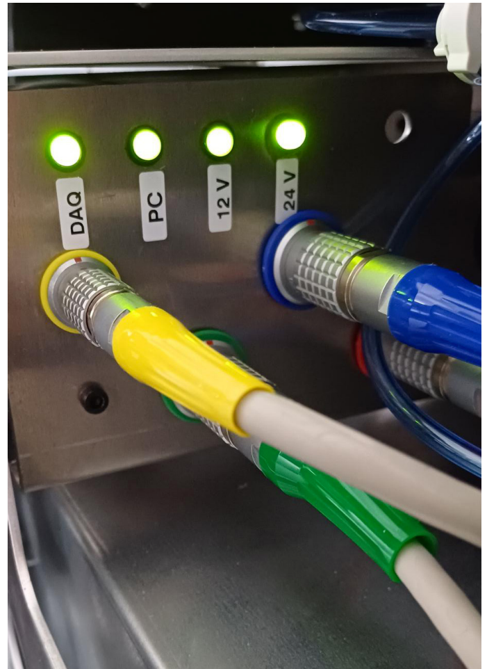
Connector panel, cable connections and indicator leds inside the case
