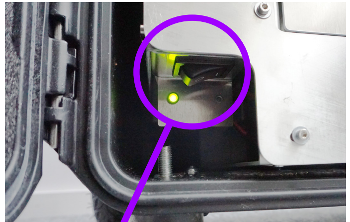
Main switch inside the case
