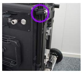
**3.** Attach the display stand to the main unit and tighten the screw. Make sure that the quick lock is closed.
