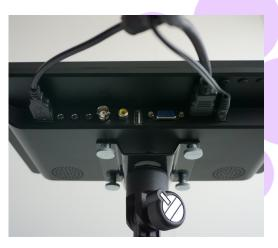
**4.** Connect the HDMI, USB and the power cable to the display.
