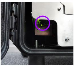
**8.** Turn ON the main switch <u>inside</u> the case. Make sure you can see the green led lights up.
