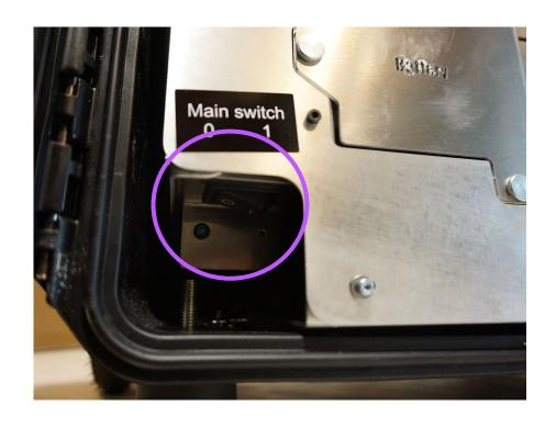
Remember to turn off the battery from the main switch inside the case before shipping the device
