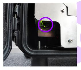
8. Turn ON the main switch <u>inside</u> the case. Make sure you can see the green led lights up.
