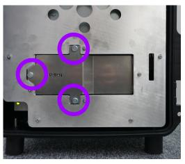
6. Connect the battery by opening the main unit cover and open the three screws.
