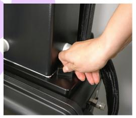
Place the measuring head to the holder at the top of the device. Remember to lock the measuring head in place with the locking knob.
