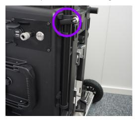
Attach the display stand to the main unit and tighten the screw. Make sure that the quick lock is closed.
