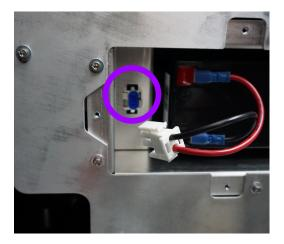
7. Remove the blue insulator part from the panel connector and attach the connectors together. Place the battery cover back and tighten the three screws.
