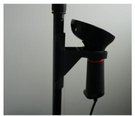
Place the barcode holder on the display stand and attach the barcode USB to the main unit.
