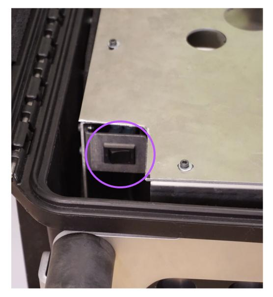
Remember to turn off the battery from the switch inside the case before shipping the device
