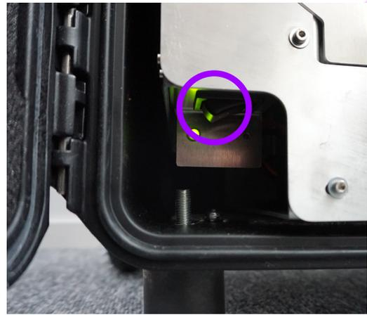
**8.** Turn ON the main switch **inside** the case. Make sure you can see the green led lights up.
