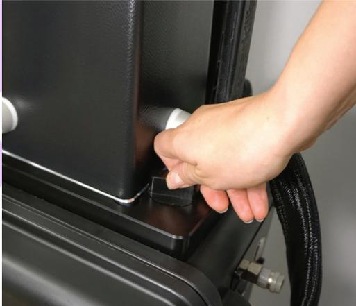
1. Place the measuring head to the holder at the top of the device. Remember to lock the measuring head in place with the locking knob.
