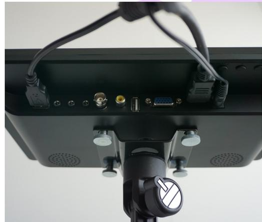
4. Connect the HDMI, USB and the power cable to the display.
