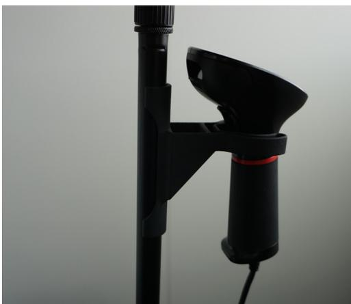
5. Place the barcode holder on the display stand and attach the barcode USB to the main unit.
