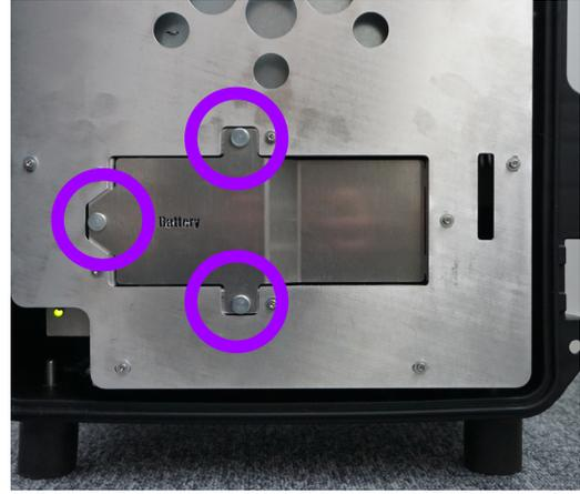
6. Connect the battery by opening the main unit cover and open the three screws.
