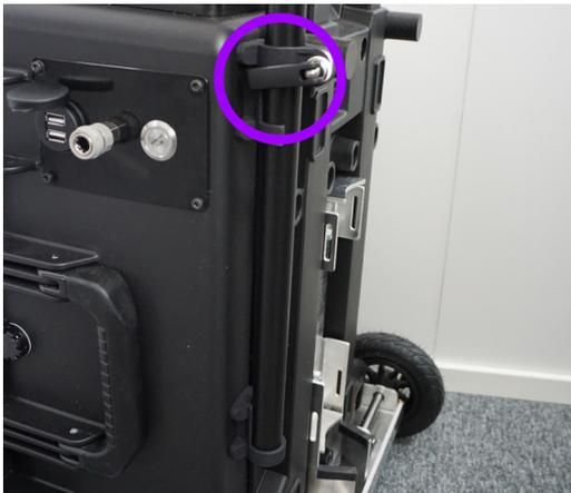
3. Attach the display stand to the main unit and tighten the screw. Make sure that the quick lock is closed.
